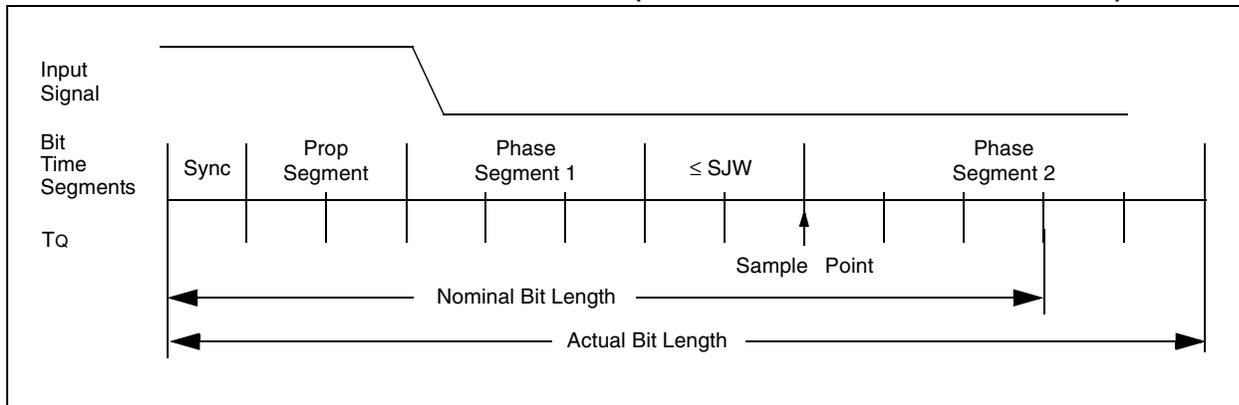
**FIGURE 23-7: SHORTENING A BIT PERIOD (SUBTRACTING SJW FROM PHASE SEGMENT 2)**
