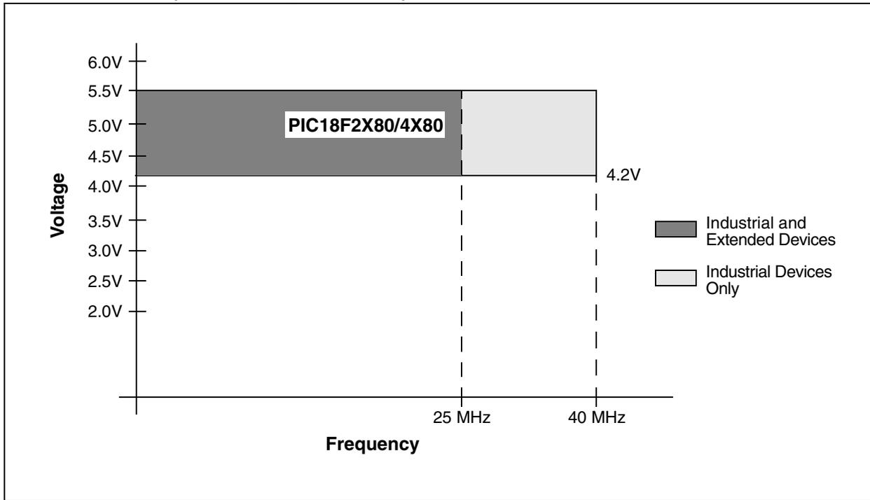
**FIGURE 27-2: PIC18LF2480/2580/4480/4580 VOLTAGE-FREQUENCY GRAPH (INDUSTRIAL)**
