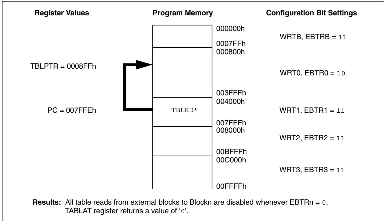
**FIGURE 24-8: EXTERNAL BLOCK TABLE READ (EBTRn) ALLOWED**
