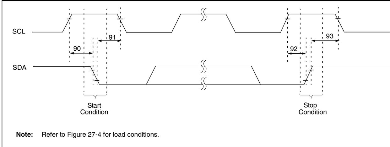
**TABLE 27-20: MASTER SSP I<sup>2</sup>C™ BUS START/STOP BITS REQUIREMENTS**
