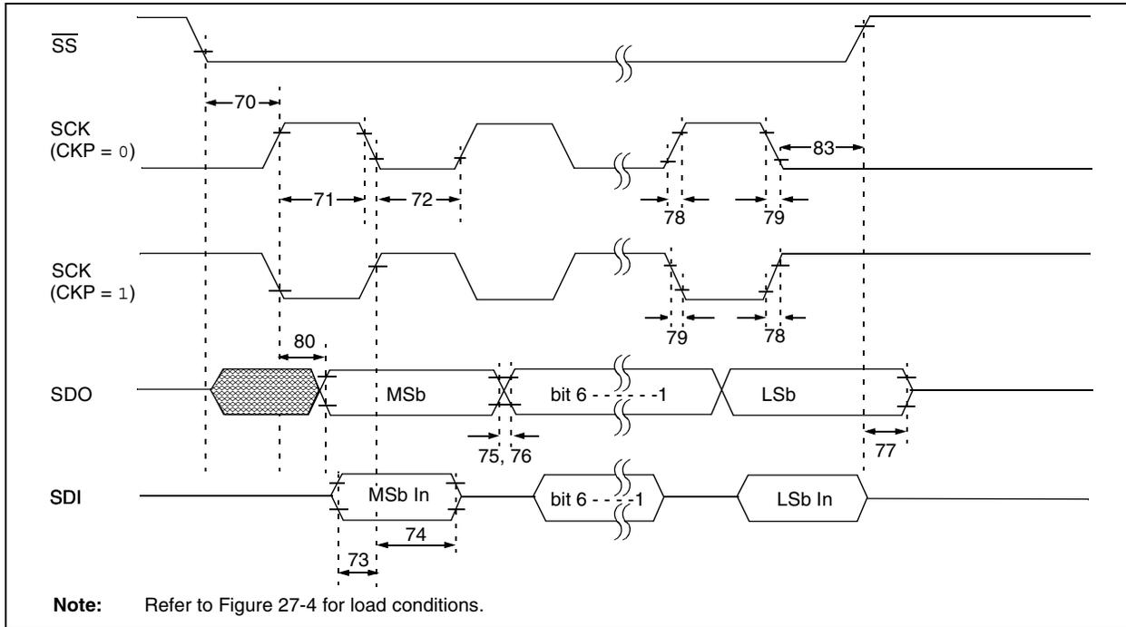
**TABLE 27-16: EXAMPLE SPI MODE REQUIREMENTS (SLAVE MODE TIMING, CKE = 0)**
