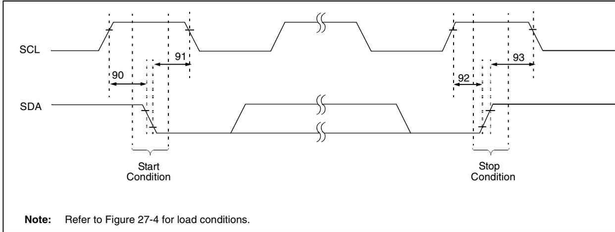
**TABLE 27-18: I<sup>2</sup>C™ BUS START/STOP BITS REQUIREMENTS (SLAVE MODE)**
