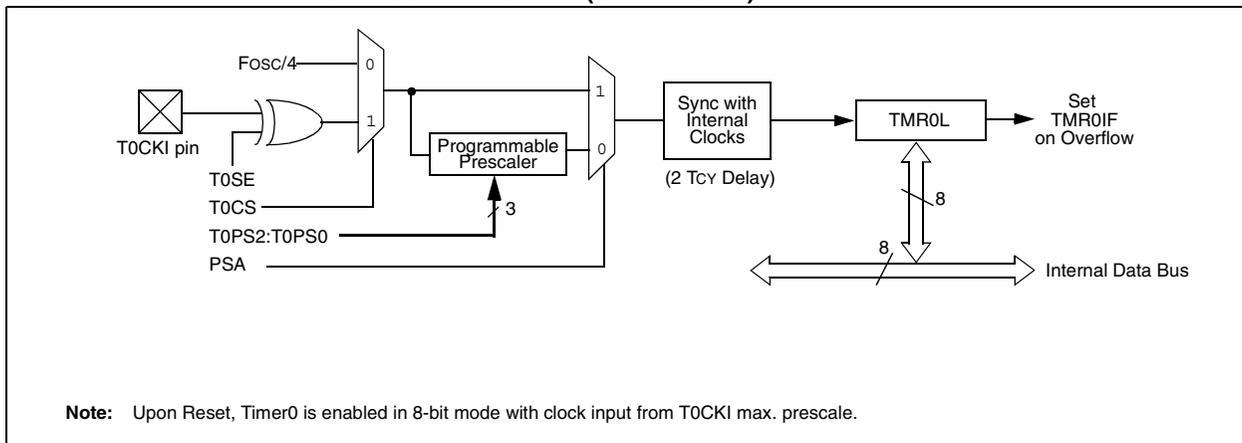
**FIGURE 11-2: TIMER0 BLOCK DIAGRAM (16-BIT MODE)**
