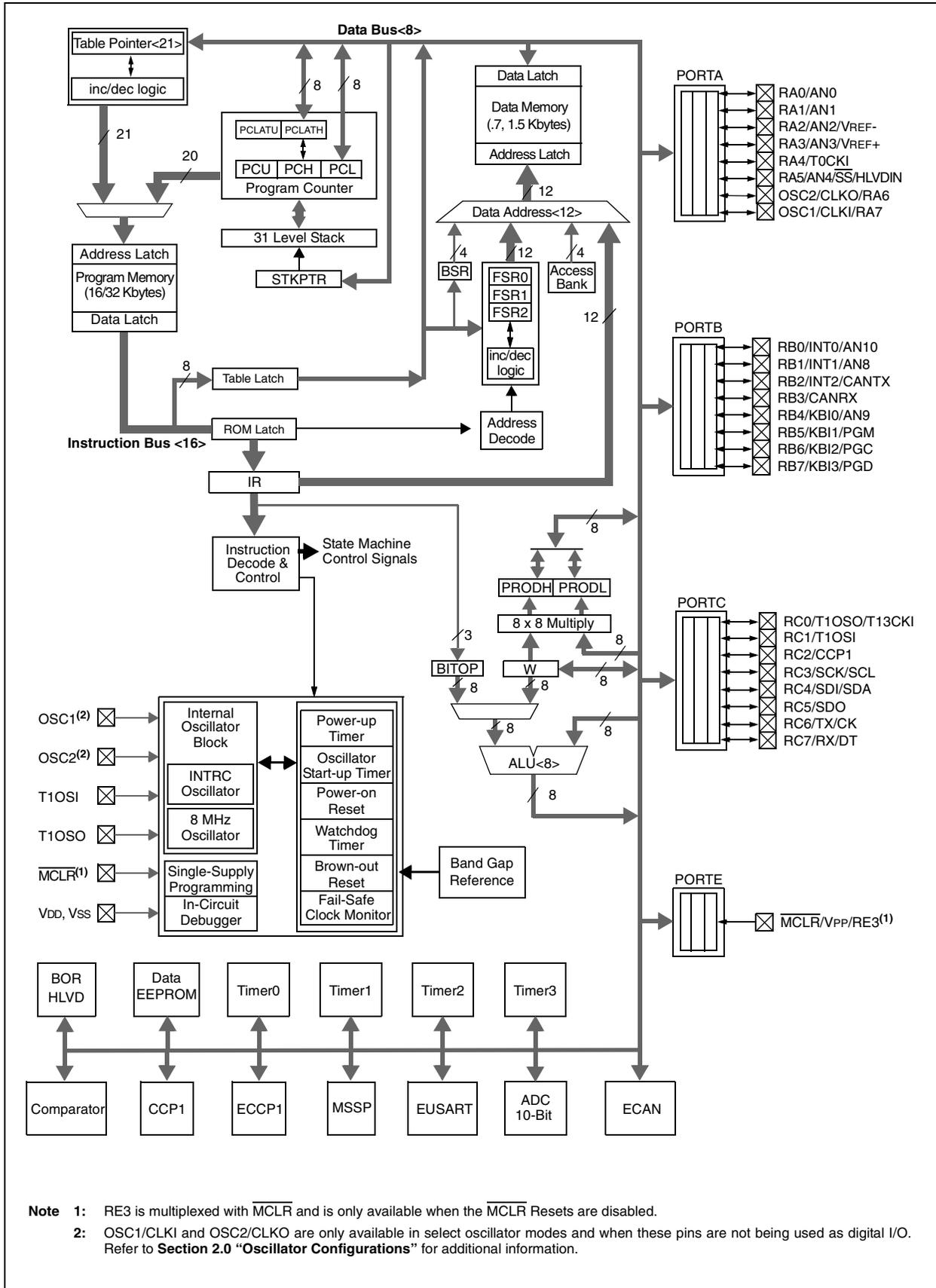
**Note 1:** RE3 is multiplexed with  $\overline{\text{MCLR}}$  and is only available when the  $\overline{\text{MCLR}}$  Resets are disabled.
