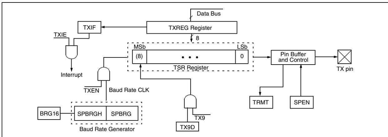
**FIGURE 18-4: ASYNCHRONOUS TRANSMISSION**
