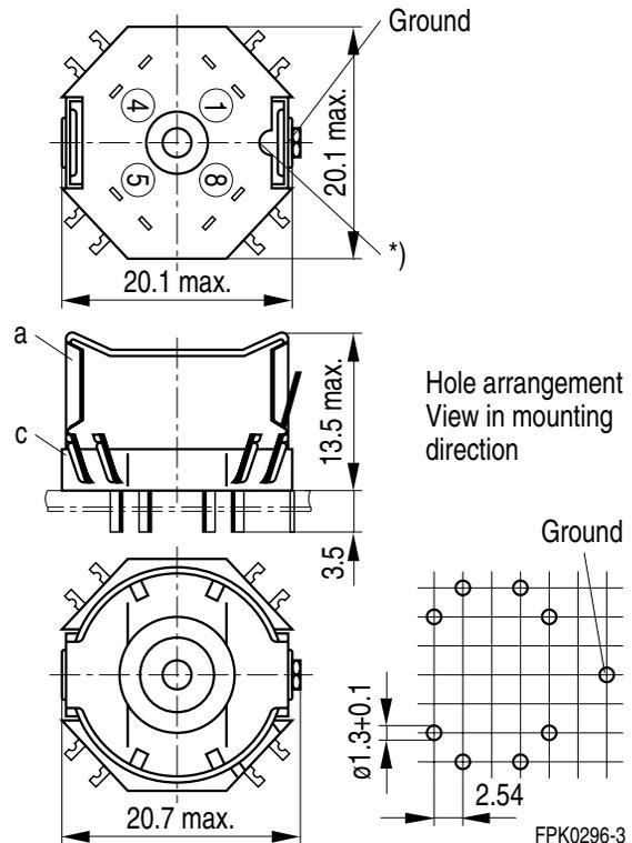
\*) This recess must be on the side of the grounding pin to ensure that the yoke locks in position.
