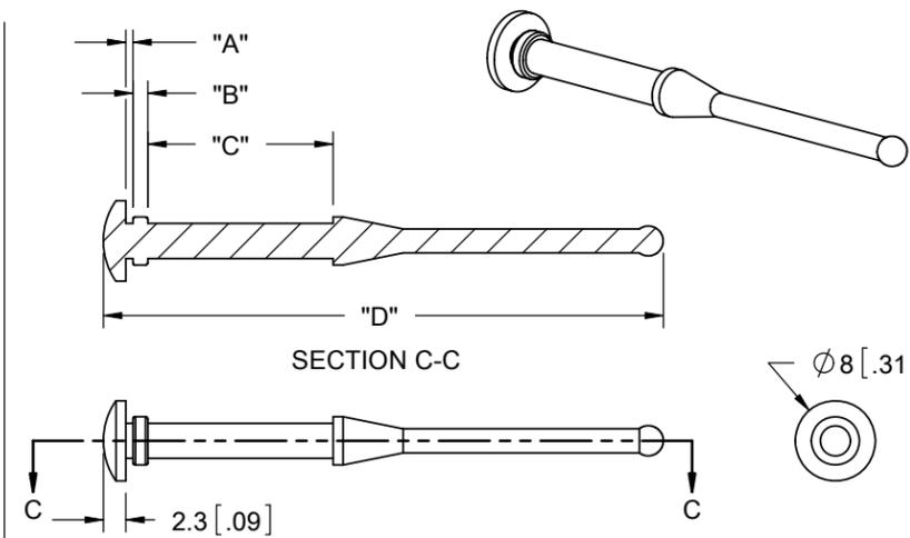
FM-5: TO PULL THROUGH A  $\varnothing 3.5 \pm 1$  [.138±.039] HOLE, WITH MAXIMUM 0.8 [.031] PANEL AND 20±0.5 [.787] FAN THICKNESS.
