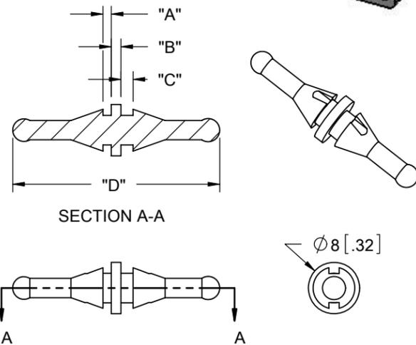
TO PULL THROUGH A  $\varnothing 5 \pm 1$  [.197±.039] HOLE, WITH MAXIMUM 1.4 [.055] PANEL AND 2 [.079] FAN THICKNESS
