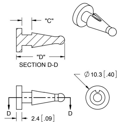
TO PULL THROUGH A  $\varnothing 5 \pm 1$  [.197±.039] HOLE, WITH 5.4 [.213] MAXIMUM TOTAL THICKNESS
