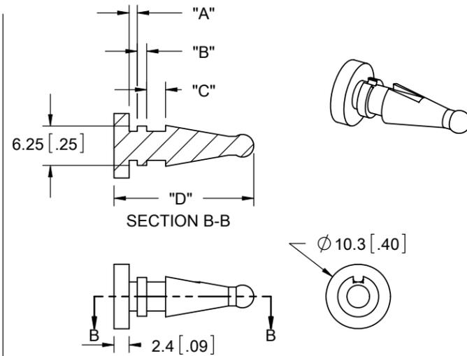
TO PULL THROUGH A  $\varnothing 5 \pm 1$  [.197±.039] HOLE, WITH MAXIMUM 1.4 [.055] PANEL AND 3.1 [.122] FAN THICKNESS
