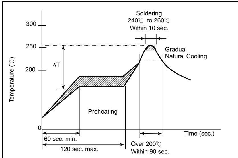
The difference between solder and chip surface should be controlled as following table. The rate of preheat should not exceed 4°C/sec and a target of 2°C/sec is preferred.
