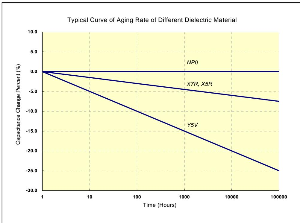
When heating the capacitors above Curie temperature (130°C~150°C) the capacitance can be re-new. So capacitance of class 2 capacitors will be complete de-aged by soldering process; subsequently a new aging process begins.
