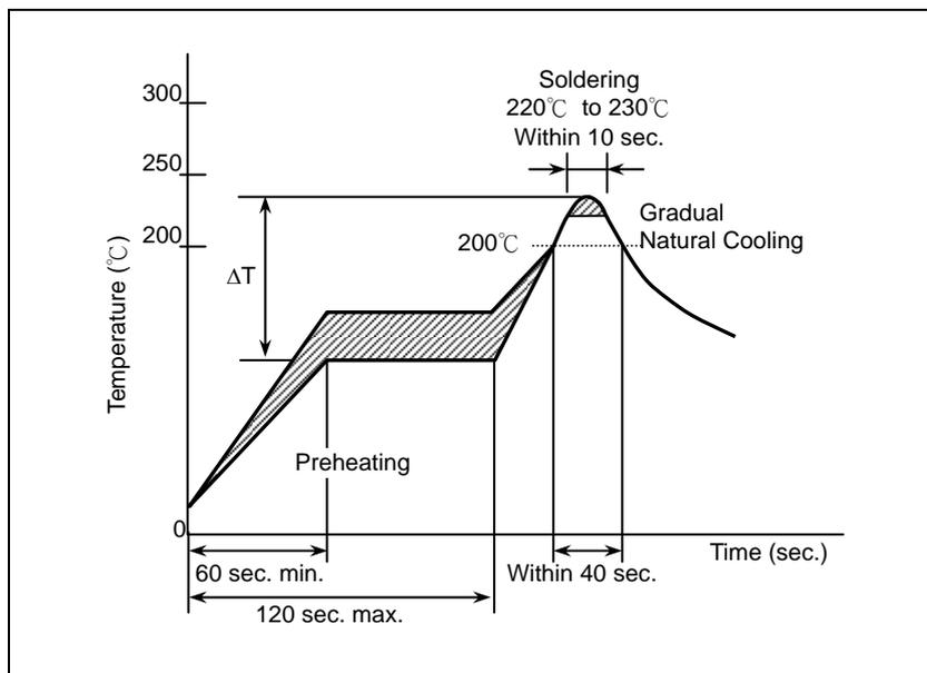
The difference between solder and chip surface should be controlled as following table. The rate of preheat should not exceed 4°C/sec and a target of 2°C/sec is preferred.
