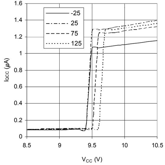
Graph 18.  $I_{QCC}$  vs  $V_{CC}$  vs Temperature (IR2156)
