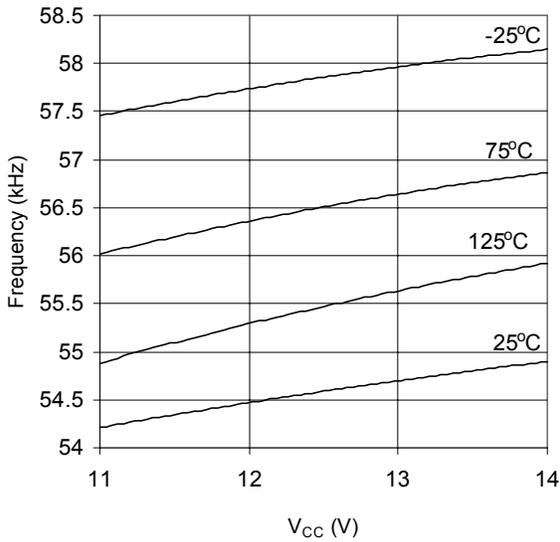
Graph 19.  $F_{OSC}$  vs  $V_{CC}$  vs Temperature (IR2156)
