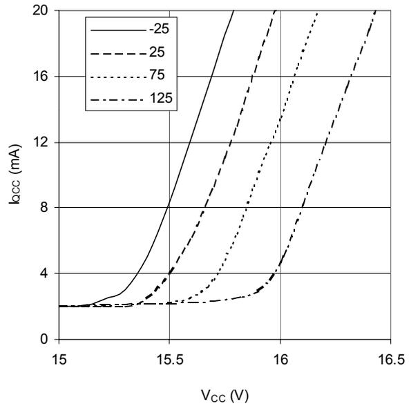
Graph 16.  $I_{QCC}$  vs  $V_{CC}$  vs Temperature (IR2156)
