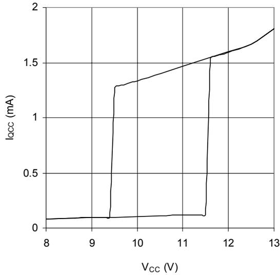
Graph 7.  $I_{QCC}$  vs  $V_{CC}$  (IR2156)
