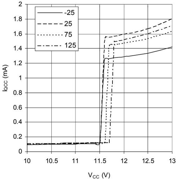
Graph 17.  $I_{QCC}$  vs  $V_{CC}$  vs Temperature (IR2156)
