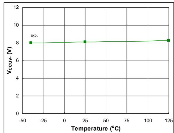
Figure 53: V<sub>CCUV-</sub> vs. temperature
