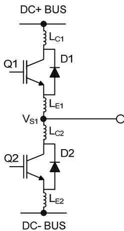
Figure 30: Parasitic Elements
