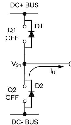
**Figure 27: D2 conducting**
