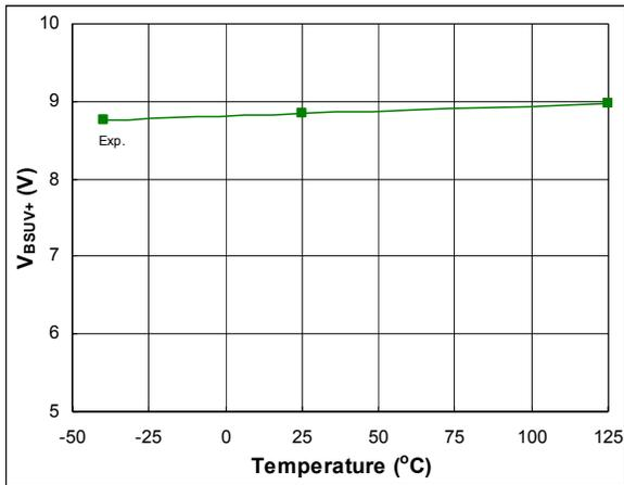
Figure 54: V<sub>BSUV+</sub> vs. temperature
