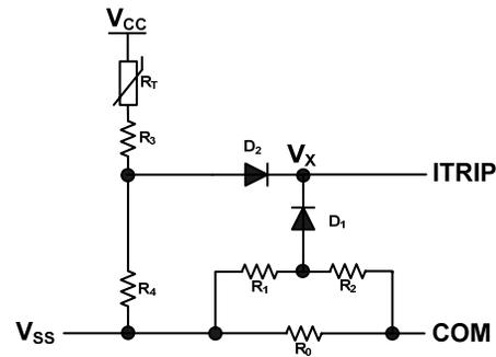
Figure 16: Using over-current protection and over-temperature protection
