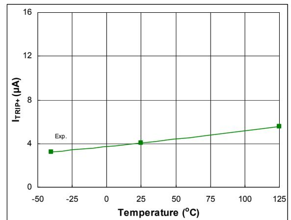
Figure 47: I<sub>TRIP+</sub> vs. temperature
