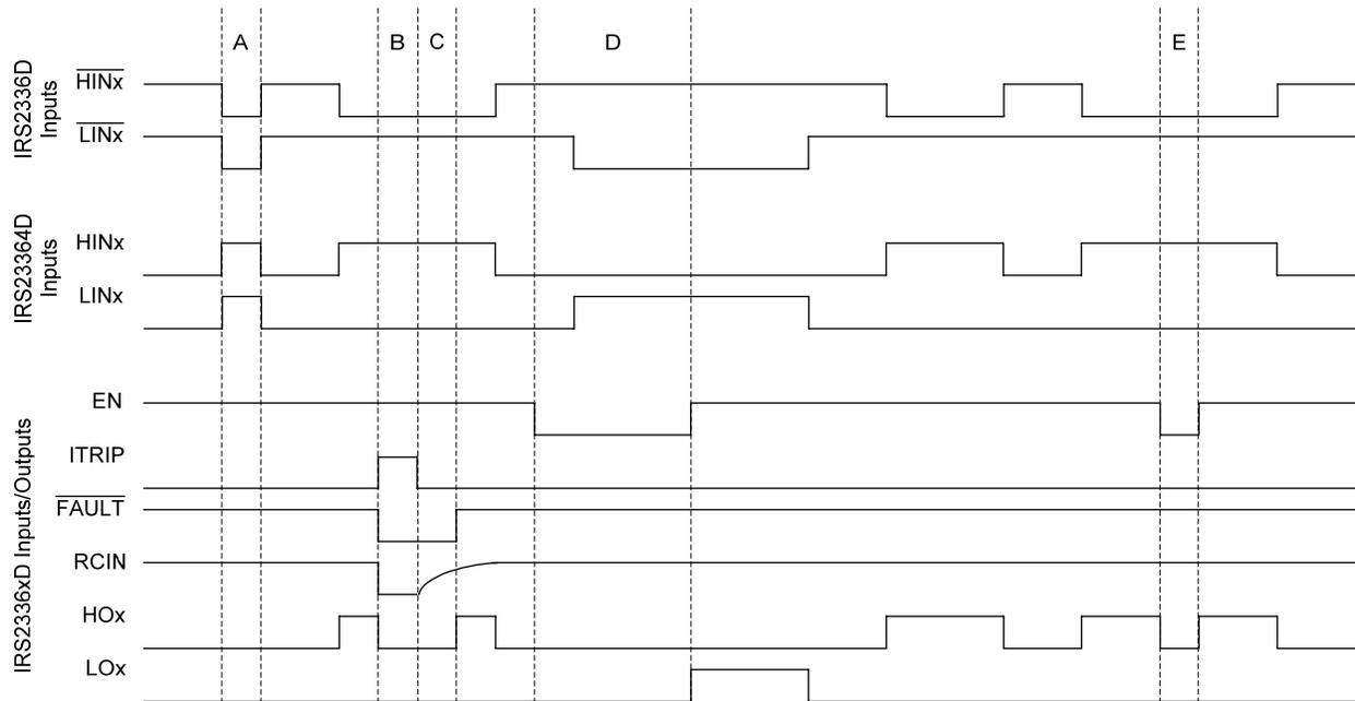
**Figure 5: Input/output timing diagram for the IRS2336x(D) family**
