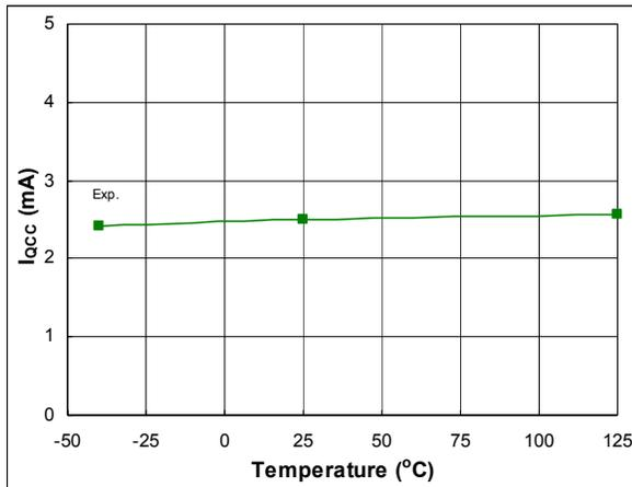
Figure 48: I<sub>QCC</sub> vs. temperature
