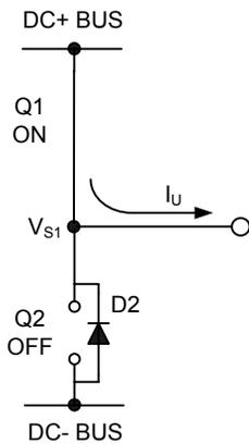
**Figure 26: Q1 conducting**
