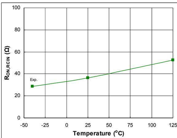
Figure 58: R<sub>ON,RCIN</sub> vs. temperature
