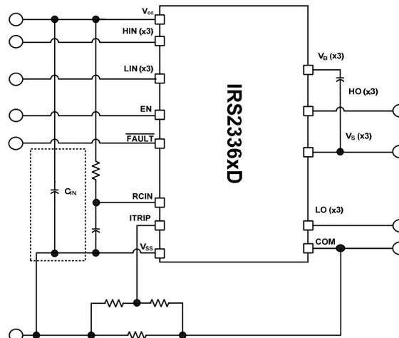
**Figure 35: Supply capacitor**
