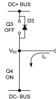
**Figure 29: Q4 conducting**
