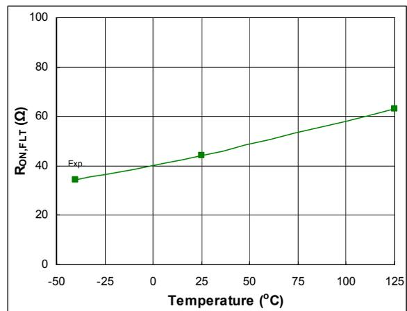
Figure 59: R<sub>ON,FLT</sub> vs. temperature
