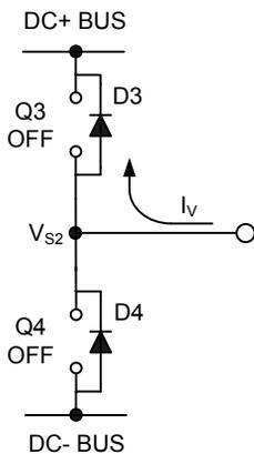
**Figure 28: D3 conducting**
