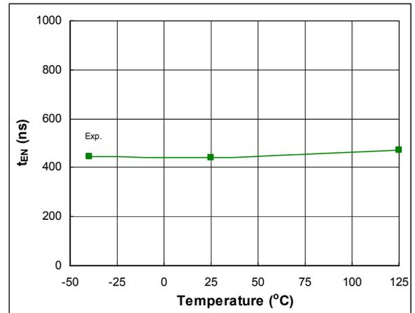
Figure 43: t<sub>EN</sub> vs. temperature
