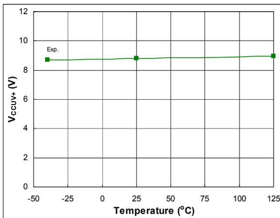
Figure 52: V<sub>CCUV+</sub> vs. temperature
