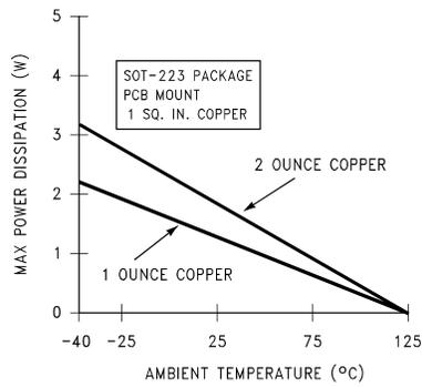
Figure 20. Maximum Power Dissipation vs. T<sub>AMB</sub> for the SOT-223 Package
