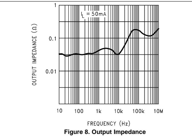
**Figure 8. Output Impedance**
