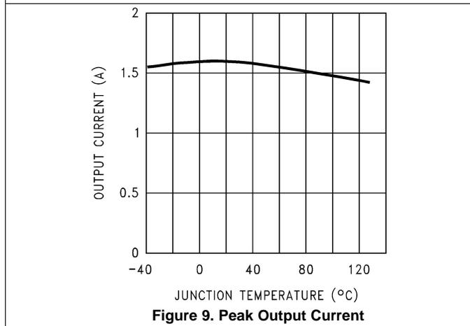
**Figure 9. Peak Output Current**
