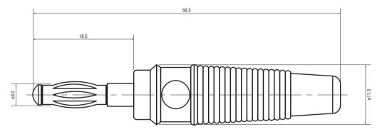
4mm Plug with the caged spring and tapering sleeve providing protection against kinking for self-assembly of test lead.
