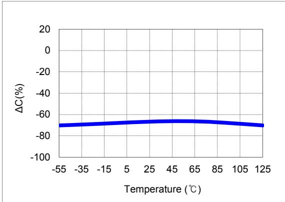
5) AC voltage characteristics (Agilent 4284A, 1kHz)
