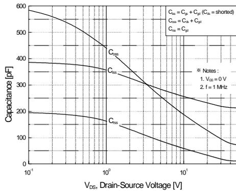
**Figure 5. Capacitance Characteristics**
