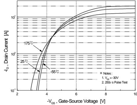
**Figure 2. Transfer Characteristics**
