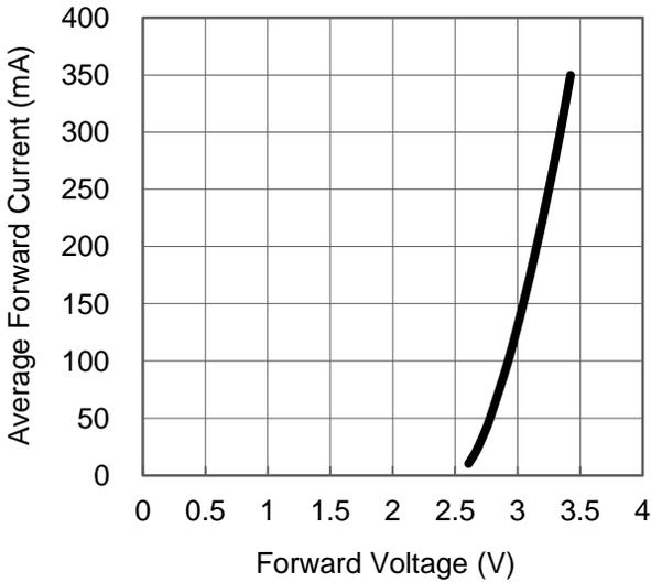
Fig 1. Forward Current vs. Forward Voltage for UV.
