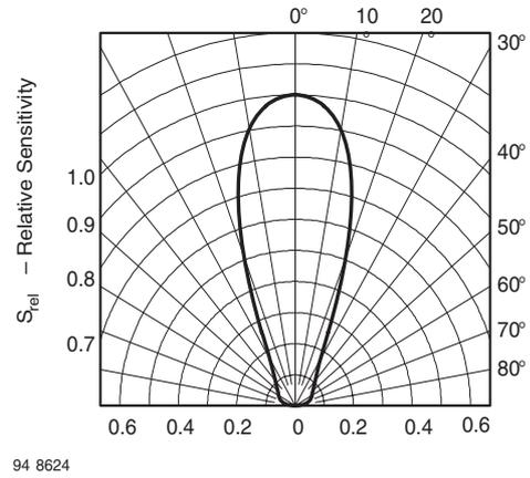
Fig. 7 Relative Radiant Sensitivity vs. Angular Displacement
