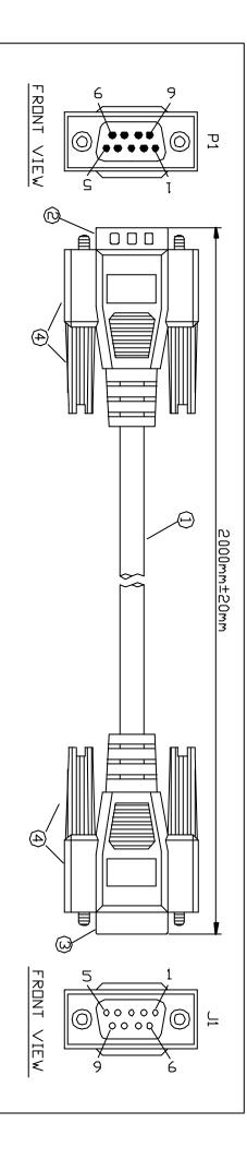
.CABLE:NO UL.,28AWG(7/0.127),TINNED AND STRANDED SHIELDIAL/MY COVERAGE ,CABLING:9C+DRAIN WIRE COPPER WIRE
